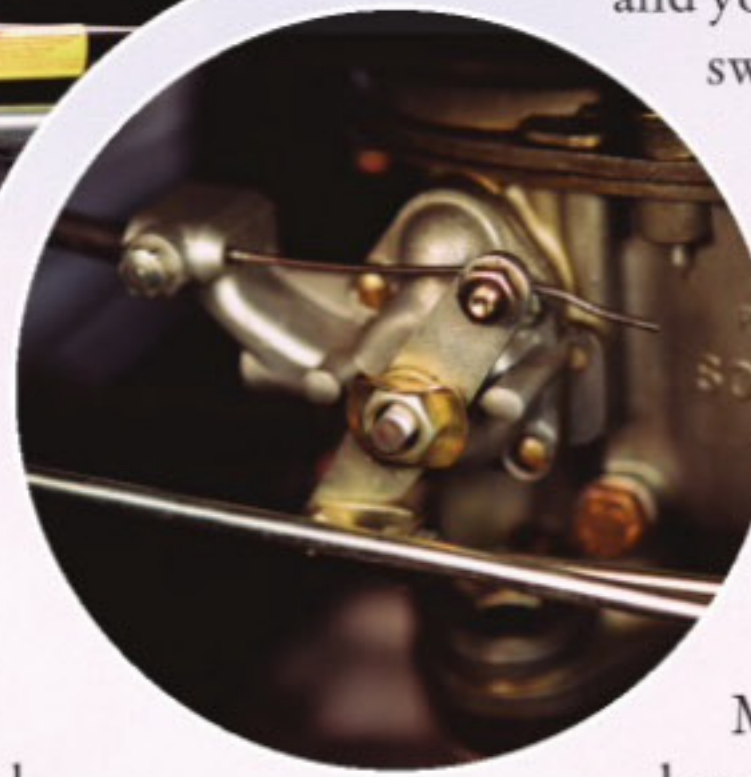
▷ Three carbs gave the 300S Roadster 148bhp.
