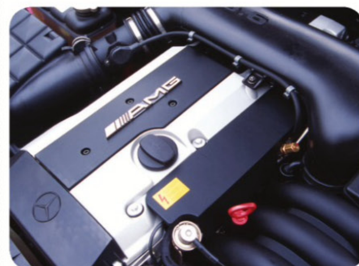
▷ 3.6-litre straight-six based on the 3.2-litre M104.
